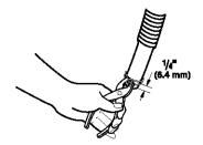
**3.** Open clamp. Twist hose back and forth while pushing onto drain connector on the side of the laundry center. Continue until hose contacts the ribbed stops on the cabinet.
