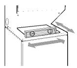
2. If the laundry center is not level, prop up the front with a wood block and adjust the feet up or down as necessary. Remove wood block and lower laundry center. Repeat this step until the laundry center is level.
