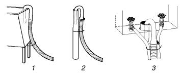
If the water faucets and the drain standpipe are recessed, put the hooked end of the drain hose in the standpipe. Tightly wrap the plastic strap around the water inlet hoses and the drain hose (3 above).
