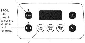
TIMER ON/OFF PAD-Used to set or cancel the PAD-Used minute timer. The minute timer does not start or stop cooking.
