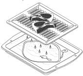
The broiler pan & the insert (some models) allows grease to drain and be kept away from the high heat of the broiler. **DO NOT** use the pan without the insert. **DO NOT** cover the insert with foil; the exposed grease could ignite.
