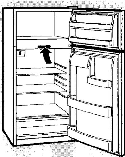
Initially, set the refrigerator control at **5** and the freezer control at **5** and allow 12 hours for the temperature to stabilize.
