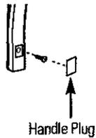
Remove the two screws holding the handle to the top of the door.
