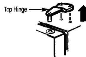
Remove the tape and tilt the door away from the cabinet. Lift it off the center hinge pin.
