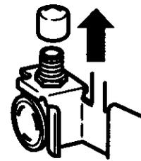
Place the compression nut and ferrule (sleeve) onto the end of the tubing as shown. On GE SmartConnect™ Refrigerator Tubing kit, the nuts are already assembled to the tubing.
