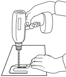
To mount anti-tip bracket to concrete or ceramic floor, use a  $\frac{3}{16}$ " (4.8 mm) masonry drill bit to drill 2 holes at the positions marked on the bracket template. Remove template from floor.
