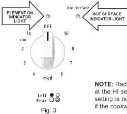
The **Element ON indicator lights** are located on the control panel above each radiant element control knob and will glow when a radiant element is turned ON. A quick glance at this indicator light after cooking is an easy check to be sure ALL surface controls are turned OFF. The **Hot Surface** indicator light located on the control panel will glow when any surface cooking area heats up and will *REMAIN ON* until the glass cooktop has cooled to a **MODERATE** level.
