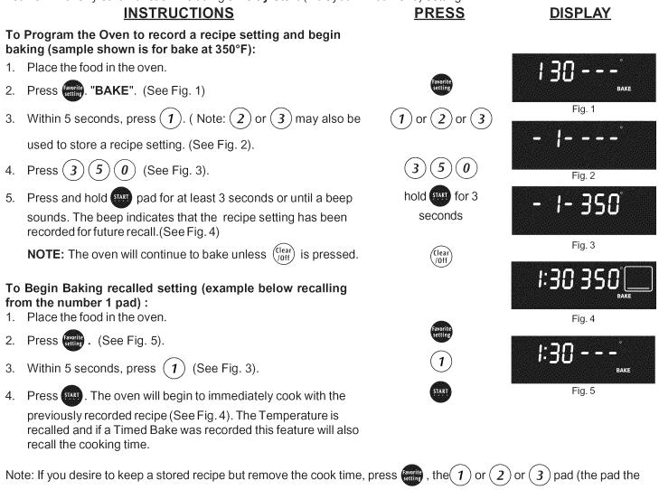
recipe is stored with). Then press  $\binom{Bake}{time}$ , press (0) and then press and hold the start pad for 3 seconds.
