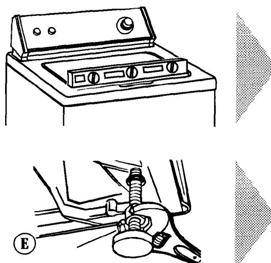
Tilt washer forward, raising back legs 2.5 cm (1 inch) off of floor to adjust rear self-leveling legs. Drop washer to floor. Check levelness of the washer by placing a carpenter's level on top of the washer, first side to side; then front to back.
