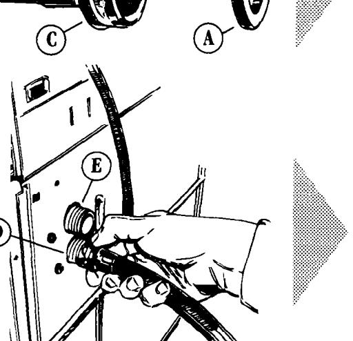
Attach hose (without adapter) to hot water (bottom) inlet valve (D) first; then second hose (without adapter) to cold water (top) inlet valve (E). Tighten couplings by hand. Then use pliers to make additional two-thirds turn.
