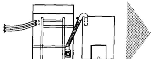
If a longer drain hose is needed, drain hose extension kit (Part No. 285702) is available from authorized parts distributors. If drain hose must be shortened, use hose kit (Part No. 285442).
