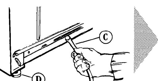
Pull firmly to remove the other end of the shipping strap (C) from the back of the washer to release self-leveling legs (D).
