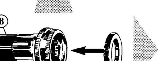
Insert a flat washer (A) into each end of the inlet hoses (B). Check that washers are firmly seated in couplings (C).
