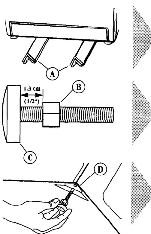
Stack two corner posts (A) on top of each other. Tilt washer backwards and slide corner posts under washer 7.6 cm (3 inches) from each side of washer as shown.
