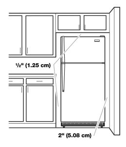
To ensure proper ventilation for your refrigerator, allow for a ½" (1.25 cm) space on each side and at the top. Allow at least 1" (2.54 cm) between back of cabinet and the wall. If your refrigerator has an ice maker, make sure you leave some extra space at the back for the water line connections.
