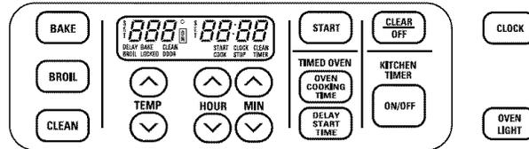
Your new touch pad oven control will allow you to set oven functions with ease. Below are the different types of functions and a description of each.
