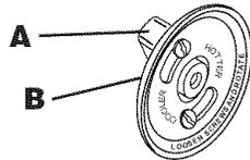
1. Turn the **OVEN TEMP** knob to **OFF** and remove it by pulling straight off.
