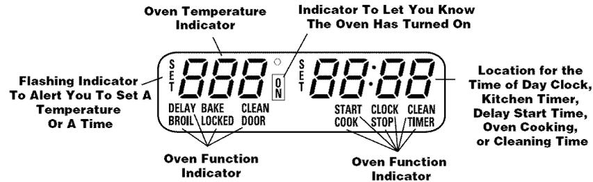
The Control Display is an easy reference for using your oven control. Below are descriptions of how the Control Display works.
