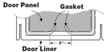
It is normal for your oven door to give the appearance of not having a good seal against the oven. This is due to the gasket. The location of the gasket on the oven door maintains a good seal and prevents any heat loss.
