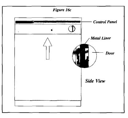
6. Unlatch door and open while supporting outer door on both sides at bottom to keep in place. Align screw holes and replace screws.
