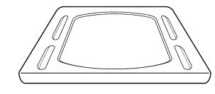
D. Remove the four screws holding the burner baffle (flame spreader) to the burner box
