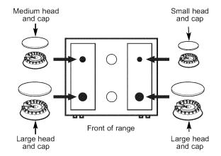
B. Make sure the slot in the burner head is positioned over the
