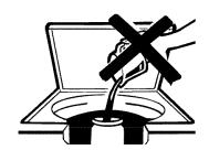
Do not pour anything into the agitator if the agitator cap or dispenser is removed.
