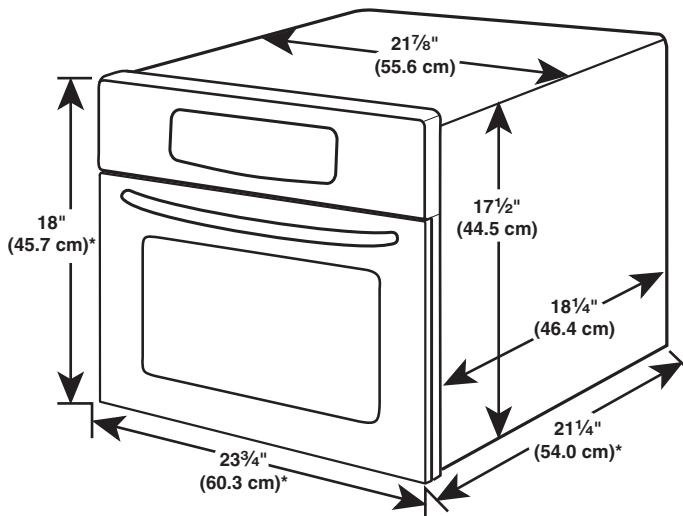
\*Measurements include front facing of microwave oven. Depth measurement also includes door handle.
