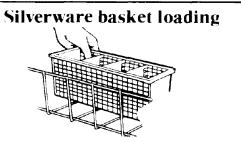
. Oad the silverware basket while it's in or out of the bottom rack. The loaded basket should be in the right front corner of the bottom rack.
