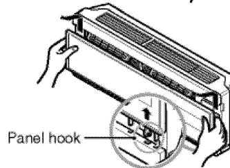
3. Come down the panel and then remove the air filter.
