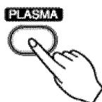
If you press the only PLASMA button, only PLASMA purification function operates. Then, fan speed is low. You can select the fan speed in four steps-low, medium, high or CHAOS.
