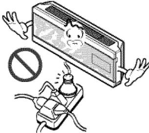
**Grasp the plug to remove the cord from the outlet. Do not touch it with wet hands.**
