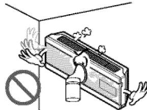
**When flammable gas leaks, turn off the gas and open a window for ventilation before turn the product on. DO NOT use the telephone or turn switches on or off.**
