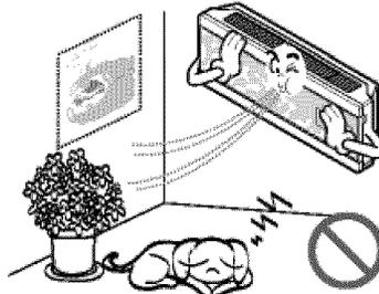
**Do not block the inlet or outlet of air flow.**
