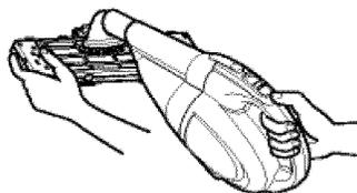
5. Relocate dried NEO plasma filter at the shade and then put in air filter.
