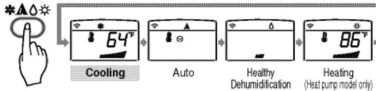
**3** Close the door of the remote controller. Set the temperature lower than the room temperature. The temperature can be set within a range of 64°F~86°F(18°C~30°C) at intervals of 2°F(1°C).
