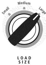
Select the load size setting most suitable for your load. Small will add a low amount of water for smaller loads and Large will add the most amount of water for large or bulky loads. Items need to move freely.
