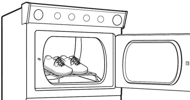
3. Place wet items on top of the drying rack. Allow space around items for air to circulate. The drying rack does not move, but the drum will rotate. Make sure items do not hang over the edges or between drying rack grille.
