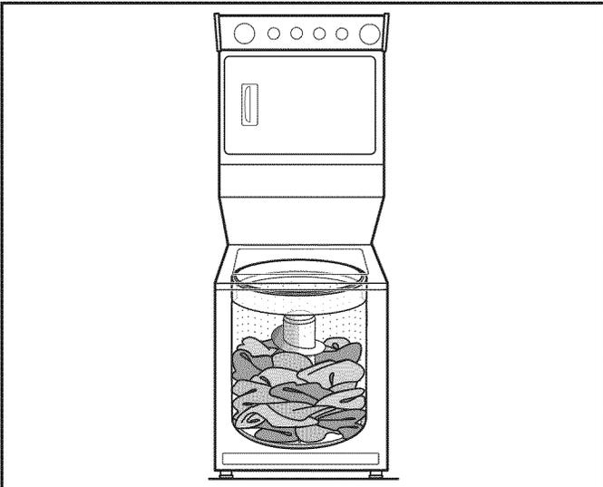
**IMPORTANT:** Do not tightly pack or force items into washer. Items need to move freely for best cleaning and to reduce wrinkling and tangling.
