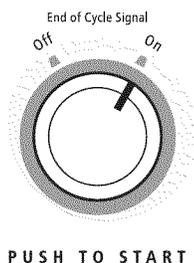
Your dryer may have an End of Cycle signal. The signal is helpful when drying items that should be removed from the dryer as soon as it stops. The End of Cycle signal is part of the PUSH TO START button and is selectable. Turn the PUSH TO START button to ON or OFF. The signal will sound only if the selector is set to ON.
