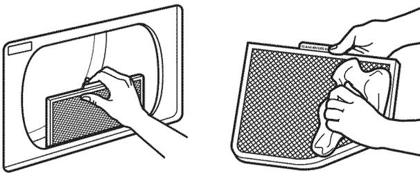
Clean the lint screen before each load. Pull the lint screen straight up. Roll lint off the screen with your fingers. Do not rinse or wash screen to remove lint. Push the lint screen firmly back into place.
