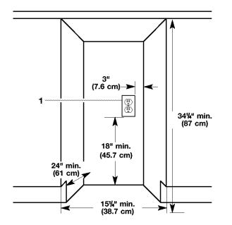
Grounded electrical outlet must be a minimum of 3 in. (7.6 cm) away from surrounding cabinets or nearby walls as shown. It can be placed either to the left or the right side of the product.
