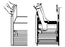
4. Place the other two corner posts on the floor to the side of the compactor. Grasp the sides of the compactor cabinet and put compactor on its side on top of the corner posts. Remove the shipping base from the bottom of the compactor.
