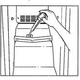
If drain becomes clogged, use a meat baster and bakingsoda-and-water solution to force the clog through the drain line.
