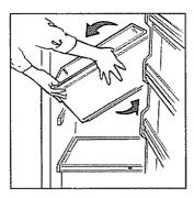
7. If tape holds bottom drawer cover to drawer supports, remove the tape. Pull drawer partway out. Reach in, push the rear of the glass up and, at the same time, back, until it clears front-corner retainers.
