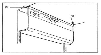
**4.** After replacing with the same size bulb, reinstall light shield.
