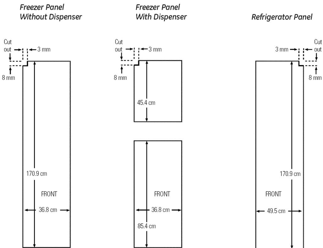
The areas at the top of the panels need to be cut out of the panels.
