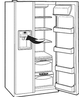
The temperature controls are preset in the factory at **5** for both the refrigerator and freezer compartments.
