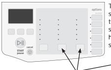
To return to factory settings, press these two buttons at the same time and hold until the signal sounds.
