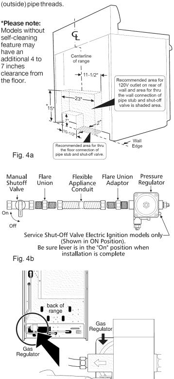
Service Gas Shut-Off Valve (shown in the "ON" position.)
