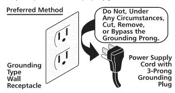
Where a standard two-prong wall receptacle is encountered, it is the personal responsibility and obligation of the customer to have it replaced with a properly grounded three-prong wall receptacle.
