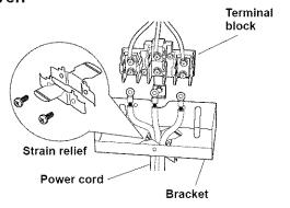
Proconduit installations only, purchase a squeeze connector matching the diameter of your conduit and assemble it in the hole. Insert the conduit through the squeeze connector and tighten. Allow enough slack to easily attach the wires to the terminal block.
