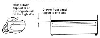
Remove and replace, making sure the rail is in the guide.
