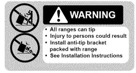
If you pull the range out and away from the wall for any reason, make sure the Anti-Tip bracket is engaged when the range is pushed back against the wall.
