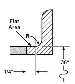
If the construction of your cabinet cannot provide a 1/4" flat area at the back of the countertop opening, consider changing the countertop to accommodate this dimension. See Alternate Construction section. If the area is not flat, excess tension may be applied to the glass cooktop, causing breakage and voiding the warranty.
