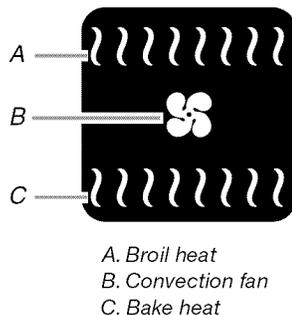
If the oven door is opened during convection roasting, the fan turns off immediately when the door is opened and turns on immediately when the door is closed. Broil and bake elements will turn off approximately 30 seconds after the door is opened. They will turn on again approximately 30 seconds after the door is closed.
