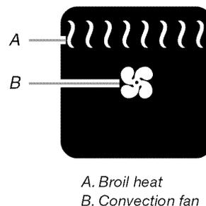
During convection broiling, the broil elements will cycle on and off in intervals to maintain oven temperature, while the fan constantly circulates the hot air.
