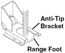
**Making sure the anti-tip bracket is installed:**
