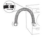
Over-the-top installation (also available with one offset elbow)
