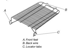
Place drying rack inside dryer drum, positioning the back wire on the ledge of the inner dryer back panel. Push down on front feet of drying rack, at the same time, aligning the locator tabs with the locator indentations in the dryer drum.
