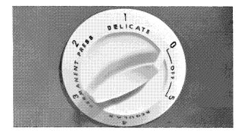
7. When the time control dial stops at 0, the load is ready to put into the spinner.
