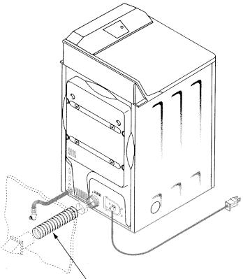
WE STRONGLY RECOMMEND THE USE OF RIGID METAL EXHAUST DUCT. IF USING FLEXABLE METAL DUCT, CUT IT TO THE PROPER LENGTH AND AVOID BUNCHING OF THE DUCT BEHIND THE DRYER.
