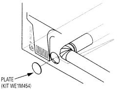
Connect standard metal elbows and ducts to complete the exhaust system. Cover back opening with a plate (Kit WE1M454) available from your local service provider. Place dryer in final location.
