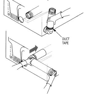
• Apply duct tape as shown on the joint between the dryer internal duct and the elbow.
