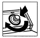
10. Pull out the Cycle Control Knob to start the washer.
