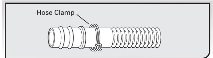
5. Push the drain hose into the connector up to the stop on the drain hose.
