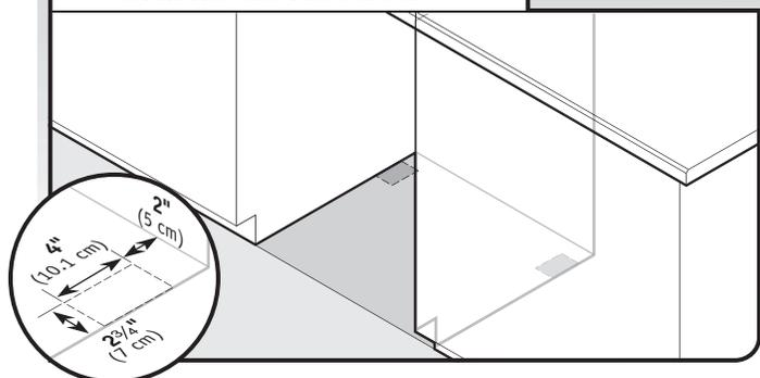
**Built-up floors:** If the kitchen floor is higher than the cabinet opening's floor - for example, the kitchen floor tile does not extend into the cabinet opening - add shims as needed in the area shown to bring the dishwasher up to 34" (86.4 cm) below the countertop.
