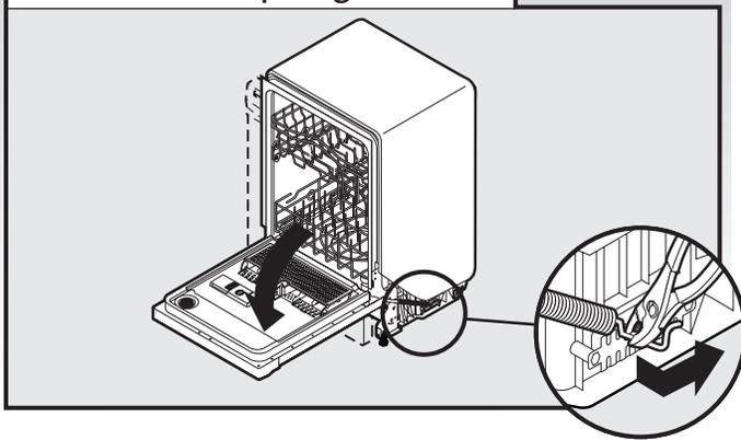
When door is unlatched, if door opens by itself, move the tensioner to a higher-numbered hole and replace the screw. Reattach door spring to rear leg.
