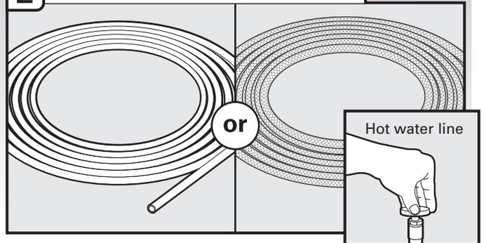
Measure overall length of copper tubing or flexible braided water supply line. Attach to the hot water line using a connection configuration that is in compliance with local codes and ordinances. The water line to the dishwasher should have a manual shutoff valve.
