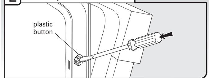
Push the plastic buttons out of the side of the tub.
