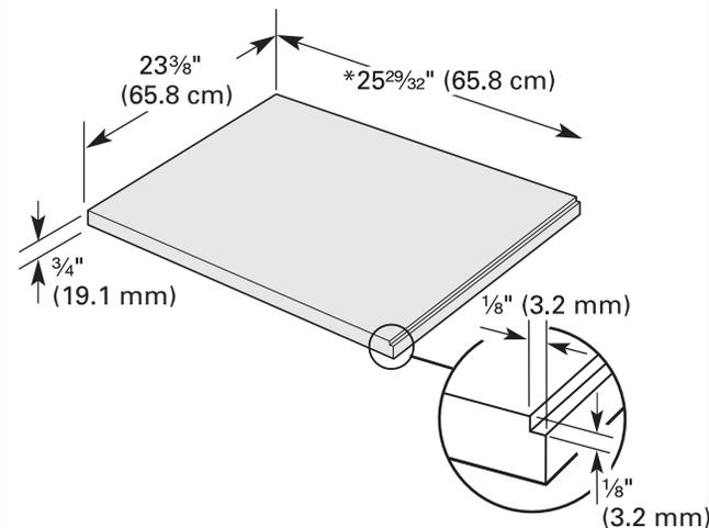
\* This dimension is for 4" (10.2 cm) toe kick. If the installation needs a higher toe kick, adjust the height of the wood panel accordingly. Not recommended for toe kicks greater than 6" (15.2 cm).
