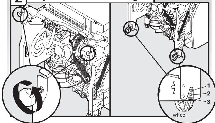
Turn both leveler legs to the same height. Put wheels in the required position determined from "Dishwasher Height Adjustment Chart."
