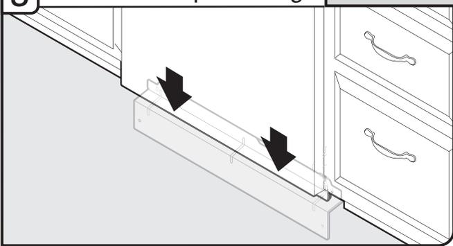
Check that the lower edge of the lower panel contacts the floor. Adjust if necessary.
