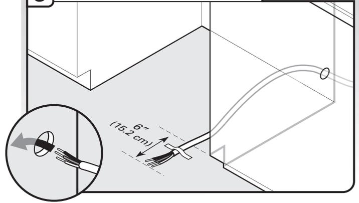
Route cable from power supply through cabinet hole (cable must extend to the right front side of cabinet opening). Tape cable to the floor in area shown. This will prohibit cable from moving when dishwasher is moved into cabinet opening.
