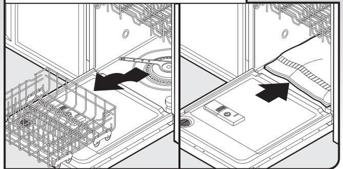
Open dishwasher door, remove lower dish rack, and place towel over pump assembly and lower spray arm of dishwasher. This will keep screws from falling into pump area when securing dishwasher to countertop.
