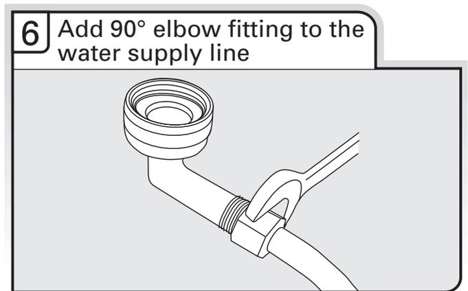
**6** Add 90° elbow fitting to the water supply line
