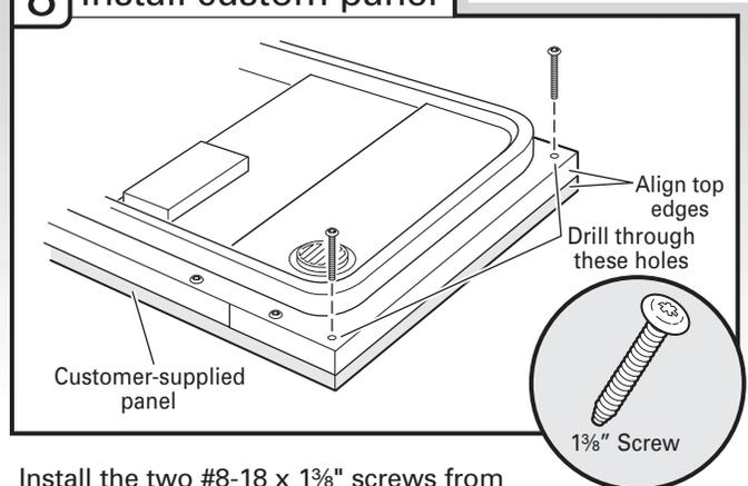
Install the two #8-18 x  $1\frac{3}{8}$ " screws from the literature package in the top corners of the inner panel. Tighten the six side screws reinstalled in Step 6.
