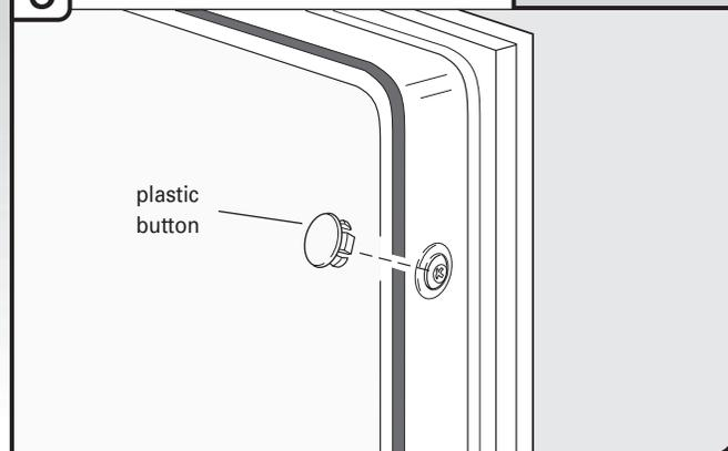
If securing with a side attachment, check that sides of door do not rub against the screw heads. If they do, dishwasher must be re-centered. When dishwasher is properly centered, replace plastic buttons.
