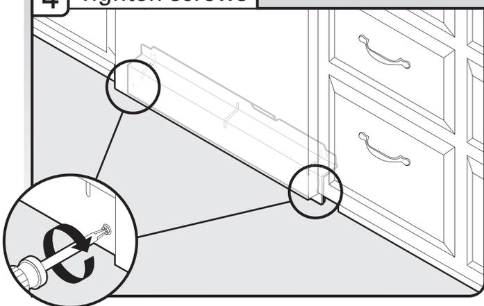
Tighten access panel screws.
