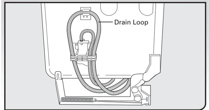
3. Place pan under end of drain hose. Pan will collect any water in drain hose.
