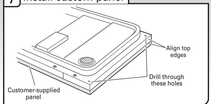
Align the top edge of the customer-supplied custom panel with the top of the console.
