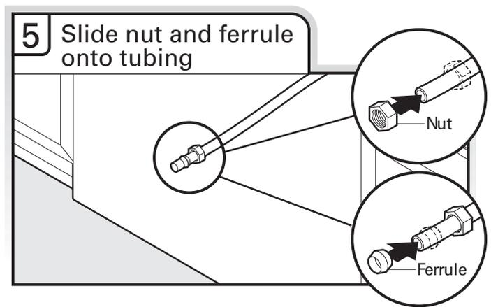
**5** Slide nut and ferrule onto tubing
