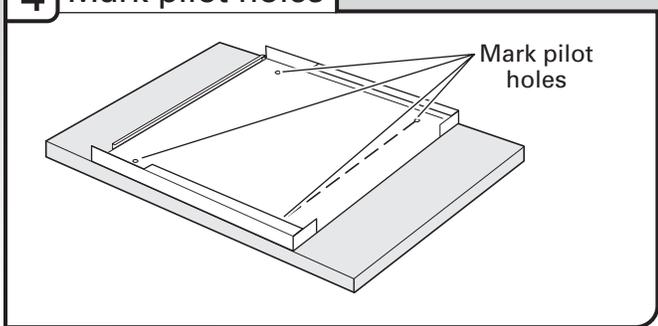
Mark all four hole locations; remove outer panel. Drill  $\frac{3}{32}$ " pilot holes  $\frac{1}{2}$ " (13 mm) deep in customer-supplied custom panel. Place the outer panel on the back of the customer-supplied custom panel; align holes.
