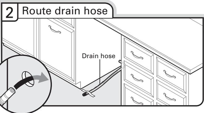
Route drain hose as shown through hole in cabinet to the front center of opening where drain connection will be made. Tape drain hose to the floor in area shown. This will keep it from moving when dishwasher is moved into cabinet opening.
