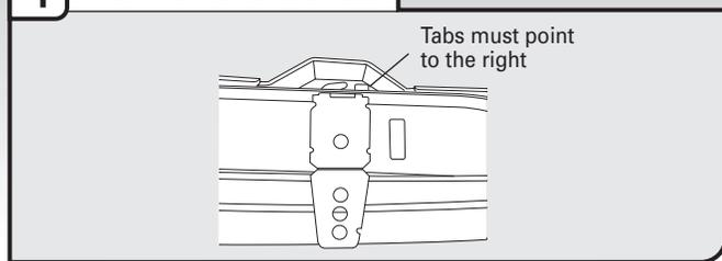
Remove the brackets from the package and place in the open slots on the left and right-hand top of the dishwasher collar as shown.
