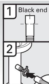
1. Connect black end of of drain hose to waste tee and cut if needed. (Do not cut ribbed section.)
