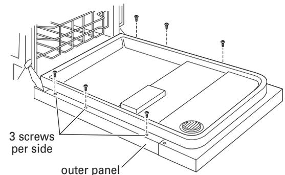
Gently set outer panel aside. Lay the customer-supplied custom panel face down on a covered, non-scratching surface.
