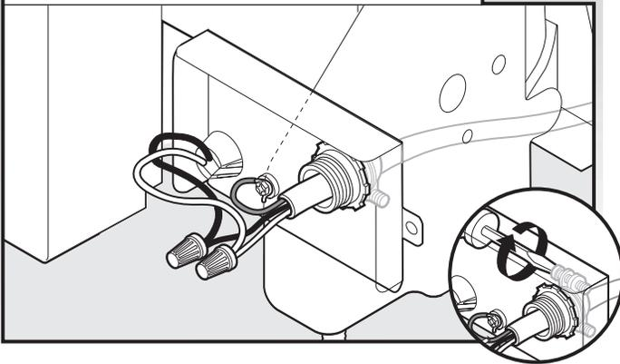
Tighten strain relief screws to secure cable.
