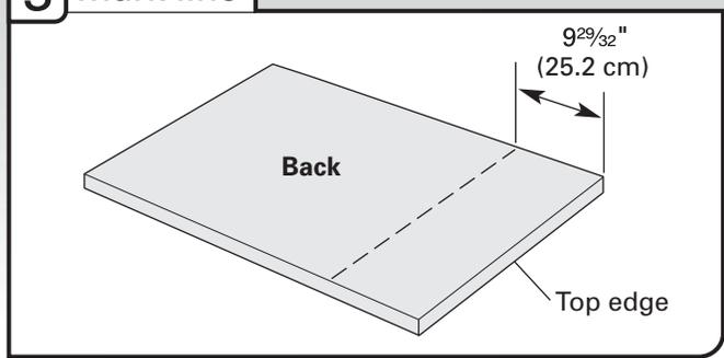
Measure  $9\frac{29}{32}$ " (25.2 cm) from top edge and mark a line on the back of customer-supplied custom panel. Position the outer panel on the back of the customer-supplied custom panel as shown, so that the top holes in the outer panel are on the line, and both panels are centered side to side.
