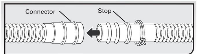
6. Use pliers to open clamp and slide clamp onto connector between stops on connector as shown.
