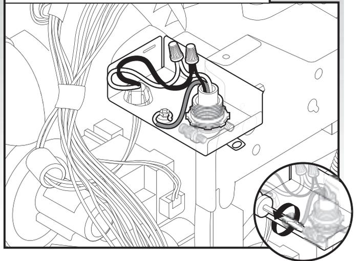
Tighten strain relief screws to secure cord.
