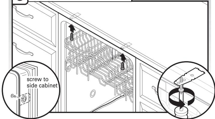
**NOTE:** Do not drop screws into bottom of dishwasher. If side mounting you must predrill ( $\frac{1}{8}$ " drill bit) pilot holes in cabinet to avoid splitting the wood before installing screws.
