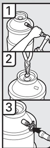
1. Using a hammer and screwdriver, knock plug into disposer.
