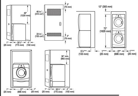
For cabinet installation, with a door, the minimum ventilation openings in the top are required.
