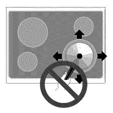
Sliding aluminum or copper clad bottom pans on the cooktop can cause metal markings on the cooktop surface. These marks should be removed **immediately** after the cooktop has cooled using the cooktop cleaning cream. Metal marks can become permanent if not removed prior to future use.
