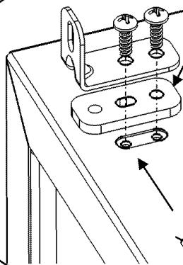
Mount Front Spacer Plate between front bracket and pedestal
