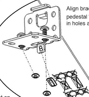
Align bracket mounting tab "B" with pedestal
