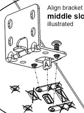
Align bracket mounting tab "A" with pedestal
