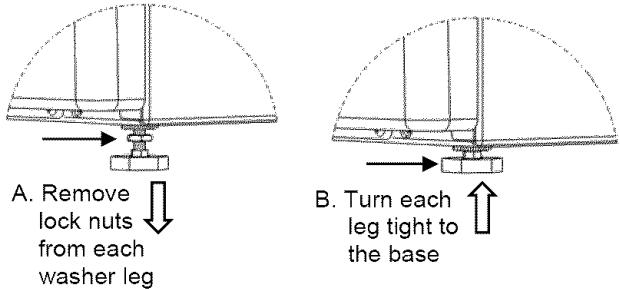
**3** On washer or dryer models with **PLASTIC LEVELING LEGS**, make sure the leveling legs are threaded fully into the base.
