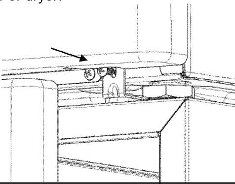
**NOTE:** If front mounting holes are not present on washer base, drill them out with a 5/32" drill bit.
