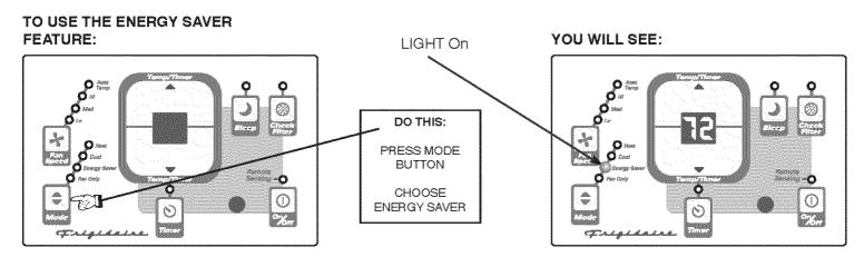
**Note:** In this mode, the fan will continue to run for 3 minutes after the compressor shuts off. The fan then cycles on for 2 minutes at 10 minute intervals until the room temperature is above the set temperature, at which time the compressor turns back on and cooling stars.
