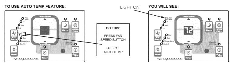
**Note:** Fan starts at High Speed and adjusts to a slower speed as the room temperature dictates. For example if the room doesn't get too warm, it will stay at the slowest speed. If the room temperature rises quickly, such as a door being opened, it will automatically go to the highest speed. The fan speeds will re-adjust back to the slowest speed as the room returns to the original set temperature. Press the fan button to adjust the fan speed manually.
