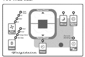
**Note:** When unit is shut off in the Heat Mode, the fan will continue to run for a few seconds to dissipate residual heat within the unit.
