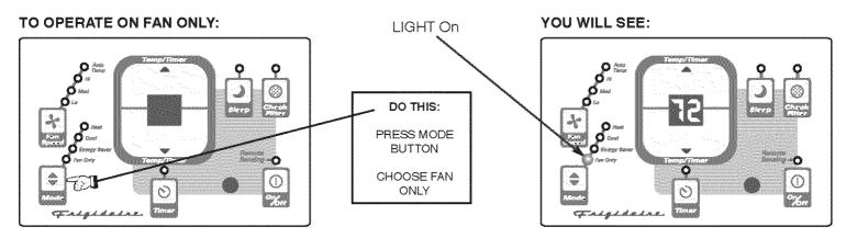
**Note:** Use this function only when cooling is not desired, such as for room air circulation You can choose any fan speed you prefer, except Auto Temp. During this function, the display will show the actual room temperature, not the set temperature as in the cooling mode.
