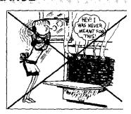
Do not obstruct the flow of combustion and ventilation a by blocking the oven vent or air intakes. Restriction of a flow to the burner prevents proper performance and increases carbon monoxide emission to unsafe levels.
