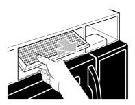
Lift the back of the charcoal filter. Slide the filter straight out.
