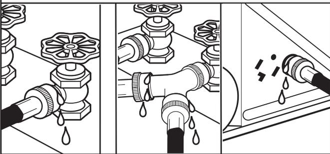
Check for leaks around "Y" connector, faucets, and hoses.
