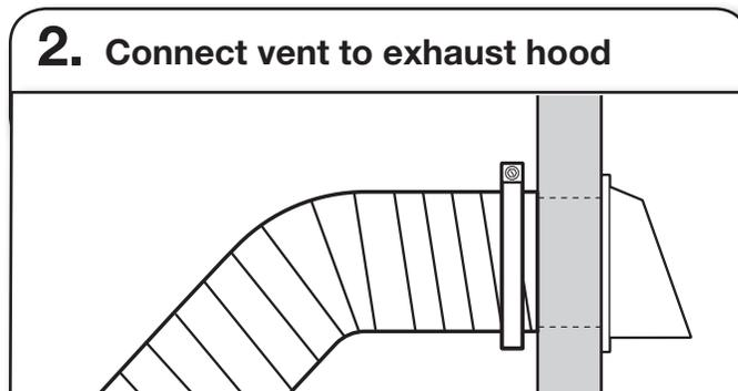
Vent must fit over the exhaust hood. Secure vent to exhaust hood with 4" (102 mm) clamp. Run vent to dryer location using straightest path possible. Avoid 90° turns. Use clamps to seal all joints. Do not use duct tape, screws, or other fastening devices that extend into interior of vent to secure vent, because they can catch lint.
