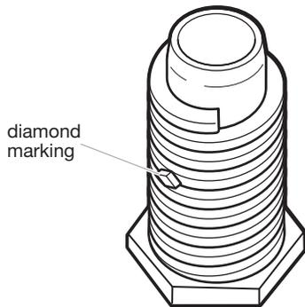
Examine leveling legs, find diamond marking. Screw legs into leg holes by hand, use a wrench to finish turning legs until diamond marking is no longer visible.
