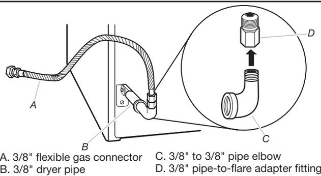
A combination of pipe fittings must be used to connect dryer to existing gas line. A recommended connection is shown. Your connection may be different, according to supply line type, size, and location.
