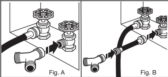
If space permits, attach the brass female end of the "Y" connector to the cold water faucet. See figure A.
