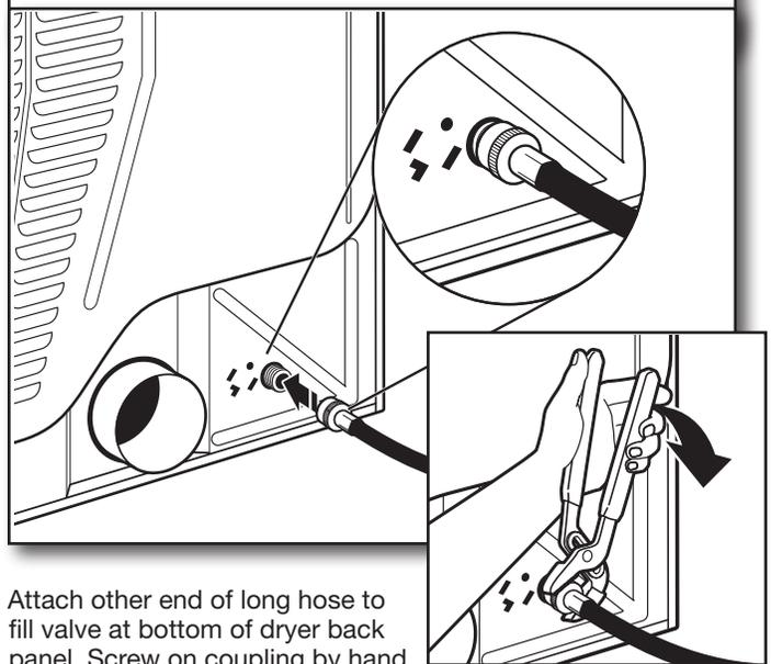
Attach other end of long hose to fill valve at bottom of dryer back panel. Screw on coupling by hand until it is seated on fill valve connector. Using pliers, tighten the couplings an additional two-thirds turn.
