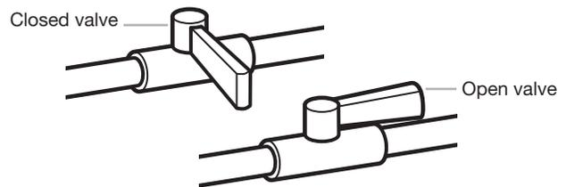
Open shut-off valve in supply line; valve is open when handle is parallel to gas pipe. Then, test all connections by brushing on an approved noncorrosive leak-detection solution. Bubbles will show a leak. Correct any leaks found.
