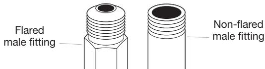
Remove red cap from gas pipe. Using a wrench to tighten, connect gas supply to dryer. Use pipe-joint compound on threads of all non-flared male fittings. If flexible metal tubing is used, be sure there are no kinks.
