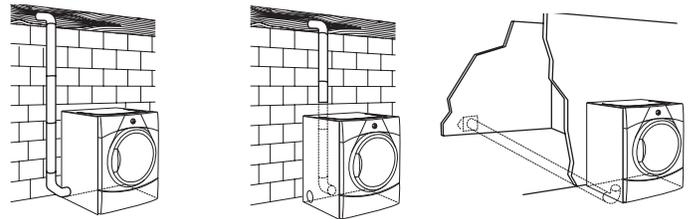
If you prefer, dryer may be converted to exhaust out right side, left side (all models except WGD9051Y), or through bottom. You must contact your local dealer to have dryer converted. Use 4-Way Exhaust Kit Part Number W10470674.
