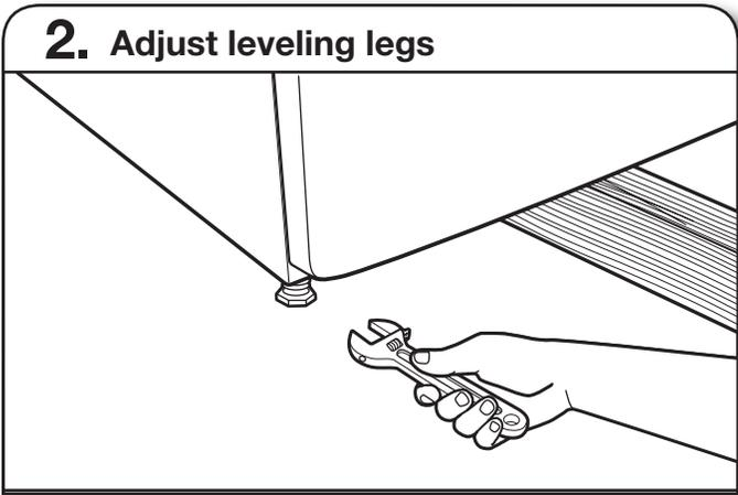
If dryer is not level, prop up using a wood block, use wrench to adjust legs up or down, and check again for levelness. Once legs are level, make sure all four legs are snug against the floor.
