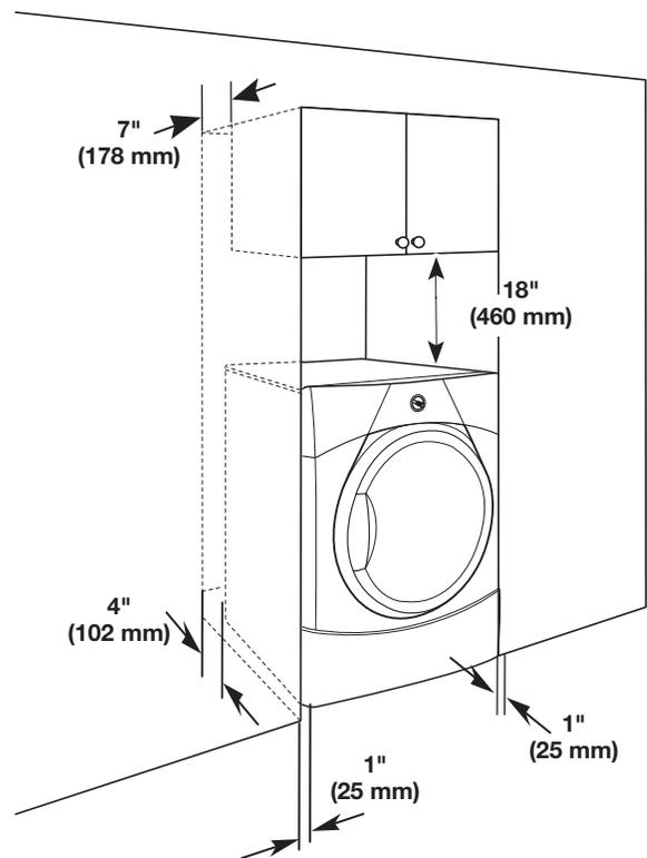
**Closet Installation (stacked washer and dryer):**
