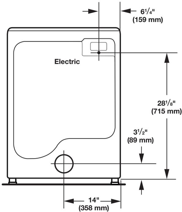
**NOTE:** Most installations require a minimum of 5" (127 mm) clearance behind dryer for exhaust vent with elbow. See "Venting Requirements."
