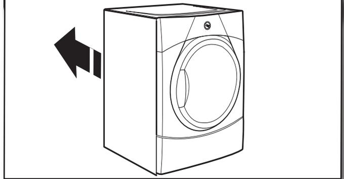
Move dryer to final location. Avoid crushing or kinking vent. After dryer is in place, remove cardboard from under dryer.
