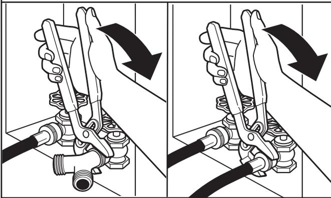
Using pliers, tighten the couplings with additional two-thirds turn.
