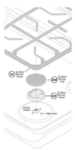
**To Remove and Replace the Surface Burner Caps and Burner Heads -**Remove in the following order: (1st) surface Burner Grates, (2nd) Burner Caps and (3rd) Burner Heads. Reverse the procedure above to replace the surface Burner Caps, Burner Heads and Burner Grates.
