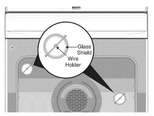
**CAUTION** Be sure the range is unplugged and all parts are COOL before replacing oven light. Wear a leather-faced glove for protection against possible broken glass.
