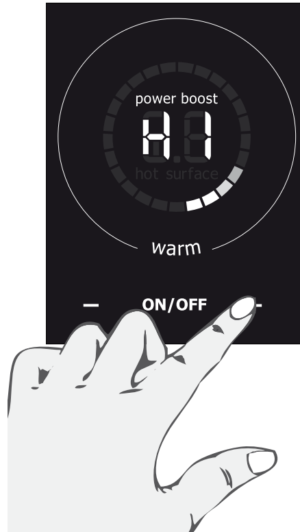
Figure 1 To set the Power Boost, press + when the zone is first turned on.
