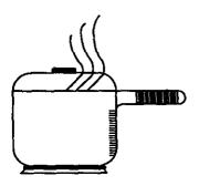
When the oven is on, heated air moves through a vent under the right rear cooktop element. This hot air may make pot handles hot or melt plastic items left too near the vent. The vent is necessary for proper oven performance. Do not block it.
