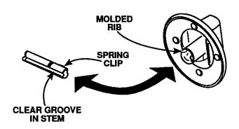
Note: Be sure to replace knobs on correct stems from which they came.
