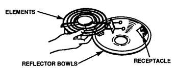
CAUTION: Do not pull element up more than 1/2" or damage to the receptacle will occur.
