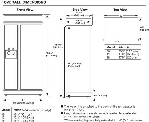
\*When leveling legs are fully extended to 11/4" (3.2 cm) below rollers, add 11/8" (2.9 cm) to the height dimensions.
