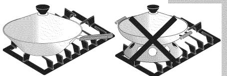
Proper use of flat-bottom wok on Surface Burner Grate Figure 2 Improper use of round-bottom wok on Surface Burner Grate Figure 3
