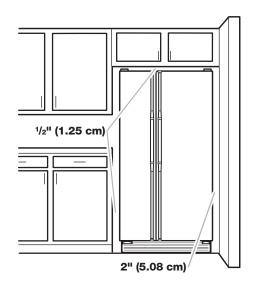
To ensure proper ventilation for your refrigerator, allow for 1/2'' (1.25 cm) space on each side and at the top. When installing your refrigerator next to a fixed wall, leave 2'' (5.08 cm) minimum on each side (depending on your model) to allow for the door to swing open. If your refrigerator has a water dispenser and ice maker, allow extra space at the back for the water line connections.
