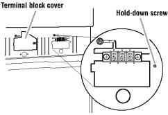
**4.** Remove the center terminal block screw. Remove the neutral grounding wire (green/yellow wire) from external grounding screw.
