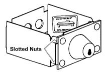
Keep a record of all coin-box key numbers. A lost key can only be replaced if ordered by key number from Sears Parts. The key number is located both on the key and behind the end panel of the coin box. If the key number is not available, the lock must be drilled out to remove the coin box.
