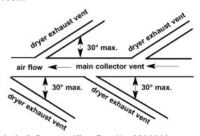
Back-draft Damper Kits, Part No. 3391910, are available from your Whirlpool dealer and should be installed in each dryer's exhaust vent to prevent exhausted air from returning into the dryers and to keep the exhaust in balance within the main exhaust vent. Unobstructed air openings are required.
