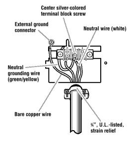
**6.** Place the hook-shaped end of the wire over the terminal block screw. The open side of the hook should face to the right. Squeeze hook end of wire together to form a loop.
