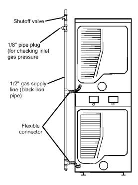
Pipe joint compounds that resist the action of L.P. gas must be used. Do not use Teflon tape.
