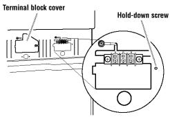
3. Attach a ¾-inch, U.L.-listed, strain relief to the hole below terminal block opening. Strain relief should have a tight fit with dryer cabinet and be in a horizontal position. Put the direct wire cable through the strain relief.
