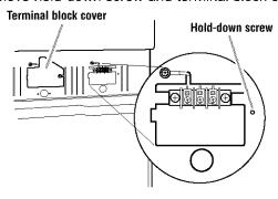
3. Attach a %-inch, U.L.-listed, strain relief to the hole below terminal block opening. Strain relief should have a tight fit with dryer cabinet and be in a horizontal position. Put the power supply cord through the strain relief.
