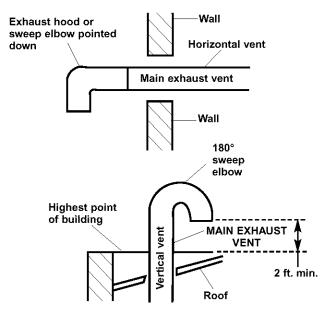
NOTE: Do not install screening or cap over end of vent.
