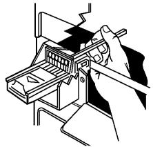
**5.** Repeat steps 3 and 4 for inserting coin slide mechanism for right side. Close the control panel.
