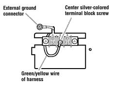
Connect neutral grounding wire and the neutral wire (white or center) of direct wire cable under the center screw of terminal block.
