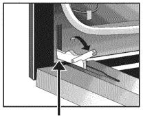
Lock engaged for door removal Figure 2
