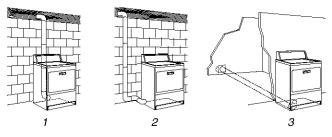
1 Standard rear offset exhaust installation
