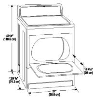
\* Most installations require a minimum 5½ in. (14 cm) clearance behind the dryer for the exhaust vent with elbow. See "Venting Requirements."
