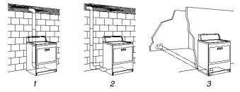
1. Standard rear offset exhaust installation
