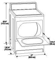
\*Most installations require a minimum 5½ in. (14 cm) clearance behind the dryer for the exhaust vent with elbow. See "Venting Requirements."
