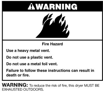
4 in. (10.2 cm) heavy metal exhaust vent and clamps must be used. DURASAFE<sup>™</sup> venting products are recommended and are available from your local Sears store or Sears Service Center.
