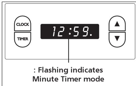
Your model may be equipped with the clock shown below. Follow the instructions to set the clock and minute timer on your range. Not all manual clean ranges are equipped with a clock.
