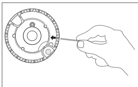
**CAUTION** Use caution when replacing the burner cap so the electrode is not damaged. This may cause a delayed ignition or prevent the burner from igniting.
