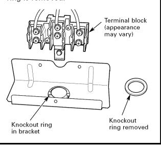
The next step if using conduit), assemble the strain relief in the hole. Insert the power cord through the strain relief and tighten. Allow enough slack to easily attach the cord terminals to the terminal block. If tabs are present at the end of the winged strain relief, they can be removed for better fit.
