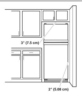
To ensure proper ventilation for your refrigerator, allow for a ½ in. (12.70 mm) space on each side. Allow 3 in. (7.5 cm) of space between overhead cabinets and refrigerator top. Allow at least 1 in. (25.40 mm) between back of cabinet and the wall. If your refrigerator has an ice maker, make sure you leave some extra space at the back for the water line connections.
