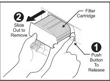
Order new filter cartridges through the dealer where you bought the refrigerator, or contact the Sears PartsDirect at 1-800-366-PART. It might be good to order some filter cartridges when you first install your refrigerator. Be sure to ask for Kenmore replacement cartridge <u>46</u>9916.
