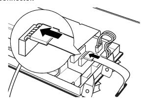
Place the ribbon and the wire from the rear cover under the strain relief on the new backsplash.
