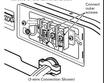
**WARNING:** Do not make a sharp bend or crimp wiring/conductor at connections.
