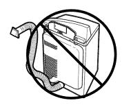
•DO NOT use excessive exhaust length. Cut duct as short as possible.
