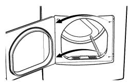
Tighten the two top screws of each hinge. Reinsert the plastic plugs on the side from which the door was removed.
