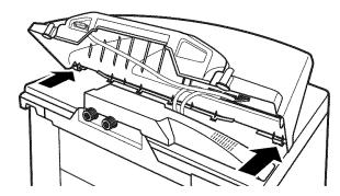
Secure the new backsplash to the washer using the two long screws removed earlier.
