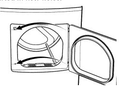
Loosen the TOP screw from each hinge on the dryer face halfway. With one hand holding the top of the door and the other hand holding the bottom, remove the door from the dryer by lifting it UP and OUT.
