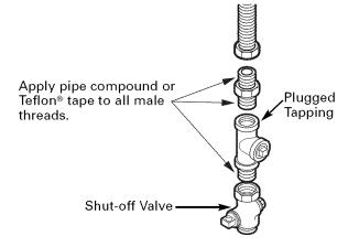
E Tighten all connections using two adjustable wrenches. **Do not overtighten**.
