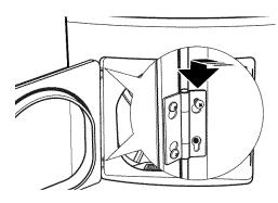
Remove the remaining screws from the side of the opening from which the door was removed. With these screws, secure each hinge at the bottom.
