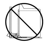
•DO NOT bend or collapse ducting. Use elbows if turns are necessary.
