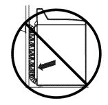
•DO NOT crush duct against the wall.
