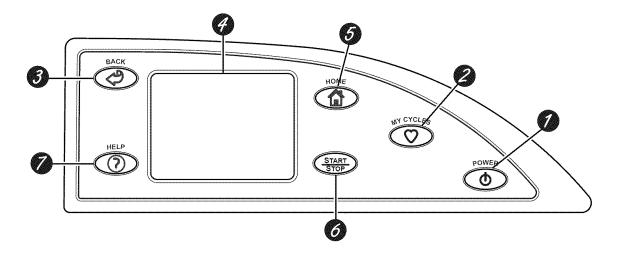
Features of the dryer control panel 1 POWER. Press to "wake up" the display. If the display is active, press to put the dryer into standby mode. You may also press the Touch Screen or any button to "wake up" the display.
