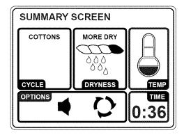
Changing the Dryness Level To change the dryness level, touch the **DRYNESS** pad on the Touch Screen; then use the arrows to select the level of dryness. Press **OK** when you have reached the desired setting.
