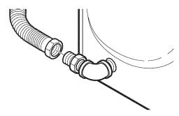
Tighten the flexible gas line connection using two adjustable wrenches.
