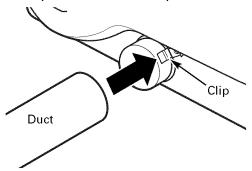
**NOTE:** We strongly recommend using rigid metal exhaust duct. If using semi-rigid metal duct, cut it to the proper length and avoid bunching of the duct behind the dryer.
