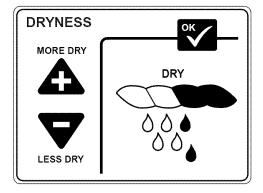
Changing the Drying Temperature To change the drying temperature, touch the **TEMP** pad on the Touch Screen; then use the arrows to select higher or lower temperature. Press **OK** when you have reached the desired setting.
