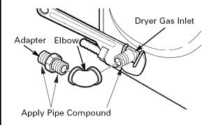
Attach the flexible metal gas line connector to the adapter.
