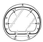
4. Use a small flat-head screwdriver to remove hole plugs in the door opening. Slide the head of the screwdriver under the cap of each hole plug, being careful not to scratch the dryer surface. Lift up. Remove the hole plugs in the door opening and insert in the opposite side.
